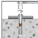
Using a wrench, expand anchor by tightening to the specified installation torque.
