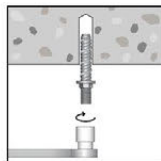
Insert anchor into hole and screw in using spanner, socket or an impact wrench. Apply constant forward pressure when driving and tighten to the specified torque.
