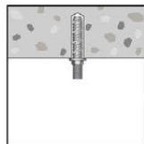
Use hand tools when removing the anchor. Do not remove with power tools if resetting the anchor.
