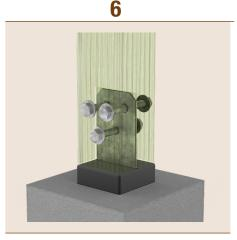
• Feed the 3 x appropriate sized bolts through the bolt holes of the centre blade and timber post. Locate washer and nuts onto the bolts and tighten. A minimum of 2 x thread pitch should extend beyond the outward surface of the nut.
