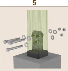
• Drill holes to accommodate appropriately sized bolts either side of the timber, meeting at the middle holes of the blade of the T Blade Bolt Down. Ensure drill through holes are horizontally levelled and perpendicular to the blade.
