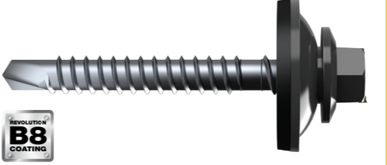
BRA Vortex RE-ROOF 6.8-10 x 60 Hex B8 (Cat 5) BRA Fixing to purlin from 1.0-5.5mm in high wind areas. SUHC868060D
